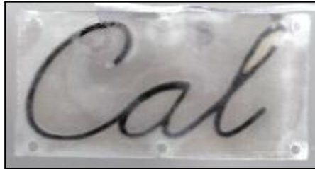
An MPI test image of nanoparticle contrast agent in a 1mm groove in plastic. Conolly hopes to increase the resolution from 3mm to 300 microns - the major remaining technical challenge.
